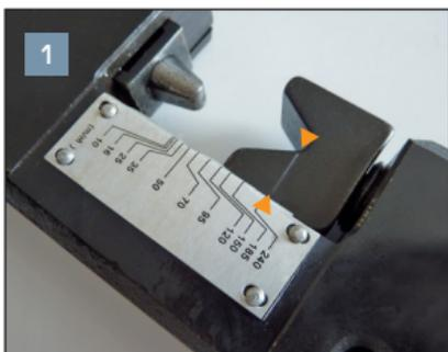
Adjust the desired cross section with the screw, making it match the mark.
