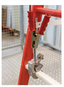
1,000V AC / 1,500V DC INSULATION TESTED TO: **100 kV** AS PER UNE-EN 61478 STANDARD
