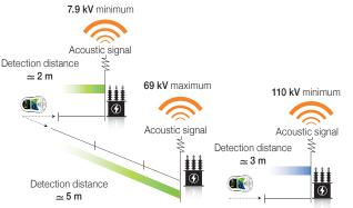
Use in Distribution / Transformation centers, Substations and AC Airlines
