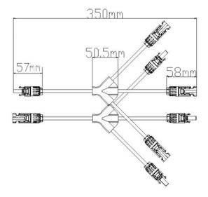
SCF/D-2TL-1500V connectors are suitable for 2-to-1, 1500 V insulation bonding.
