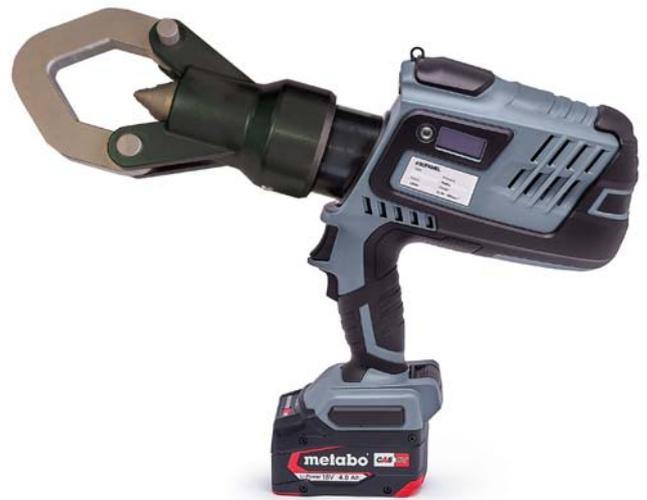
Supplied with a carrying case and a rubber hammer to free the punch, which may become temporarily stuck in the connector during deep punch crimps due to aluminium deformation.
