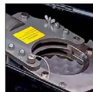
The KH-140-VOLTCUT model is a battery-powered hydraulic cutting tool designed for precise and safe cutting of copper and aluminium cables, including armoured cables and live cables up to 220 kV.
