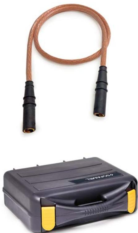
The KS-2FB-05016 kit is designed for temporary current by-passes, provisional bridging, and measurement operations in low-voltage systems. It includes a flexible 50 mm<sup>2</sup> shunt cable with female bayonet connectors, protected with Santoprene insulating sleeves, and supplied in a rigid carrying case.
