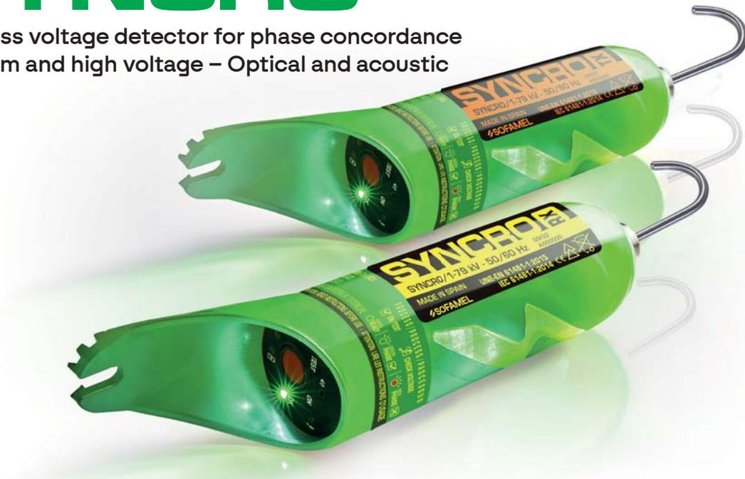
Wireless detector for phase concordance verification in electrical networks. It allows the monitoring of all types of three-phase networks from 1 to 79 kV. The absence of a connecting cable eliminates all hazards associated with its use and allows operation in high-temperature environments. Measurement through obstacles such as walls, doors, etc. is possible. Guaranteed detection distance of up to 50 m.
